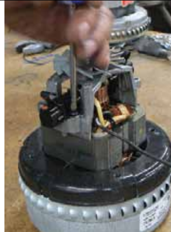
Remove brush clamp screws with a Phillips screwdriver.
