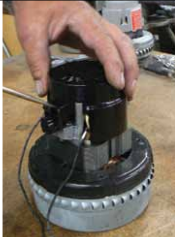
Remove the cooling fan cover.
