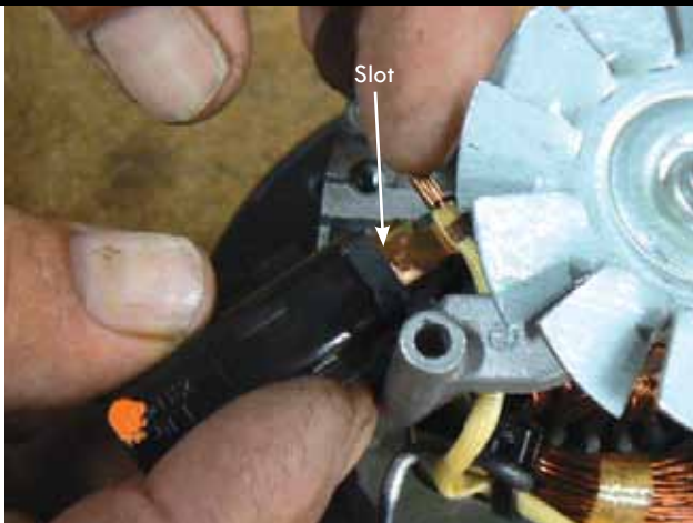
Take your new replacement brush and push the flat-brass terminal into the slot between the brush nylon (plastic casing) and the brass tube.
